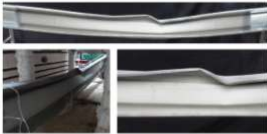
Fig 3.6 Failure mode of 2 sigma beam (L. Laim et al. (2015)).
